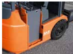
Low lift out battery extraction
